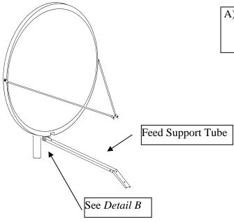
A). Mount feed support tube between the feed support brackets with [2] of (items: 8, 5, 6, 7).
