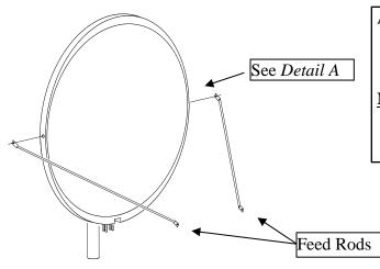
A). Attach feed rods to reflector with (items: 3, 6, 7) and with [2] of (item 5).
