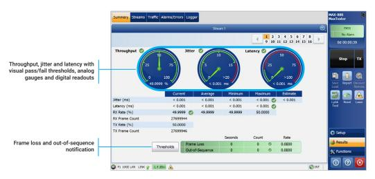
The analog gauges are lined with **green** and **red** regions to represent the expected thresholds.
