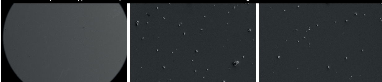
Molecular sieve particles applied from suspension onto carbon surface with Glow Discharge
