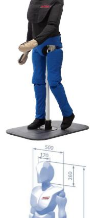
Figure 1: Dimensions compliant with ACEA specifications
