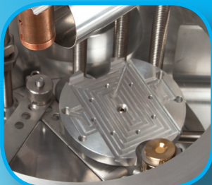
Specimen stage in position. The quartz crystal and holder of the optional film thickness monitor (FTM) locate into a recess in the stage and can be angled towards the evaporation source
