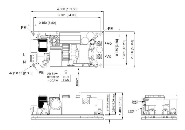
Input connector (L, N): TAIWAN KING PIN TERMINAL PVHI series. Mate connector: JST Housing VHR series or equivalent.
