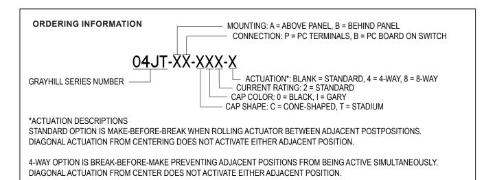
8-WAY OPTION ALLOWS ACTIVATION OF TWO ADJACENT POSITIONS DIRECTLY FROM CENTER WITH DIAGONALLY ACTUATION
