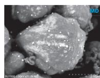
Simultaneous image acquisition for surface micro-structural information (UD), surface coating (MD), and overall topographic information (LD). Acceleration voltage: 1 kV
