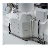
left: external view of the specimen chamber featuring . 18 accessories ports
